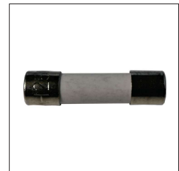
531414 G ceramic fuse 5x20 mm T6.3A H 250V
